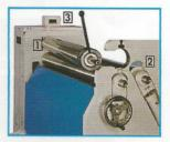
Top roll swivel out mechanism.
