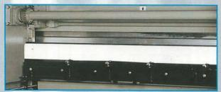
• Bottom Die/Table Hydraulic Support, ensure bent workpiece in straight alignment.
