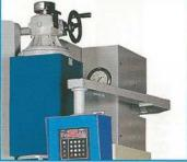
• Power Bending Angle (Depth Positioning) setting device with manual micro adjustor and readout display control panel.
